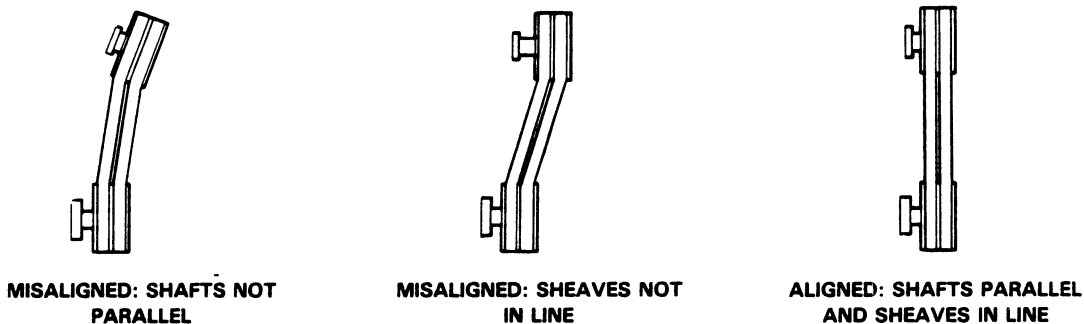
Figure 7. Alignment of V-Belt Driven Pumps
