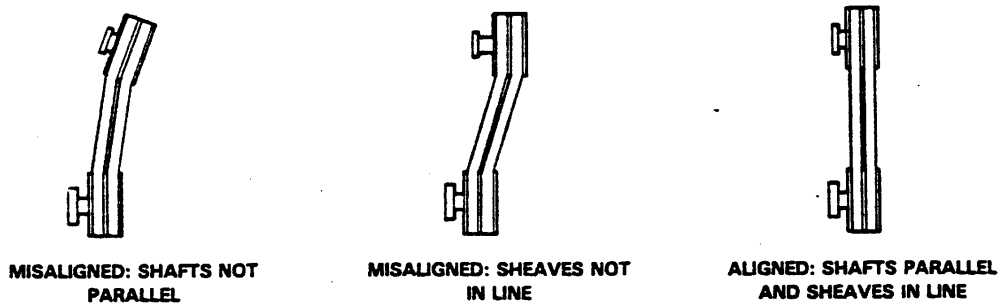
Figure 3c. Alignment of V-Belt Driven Pumps
