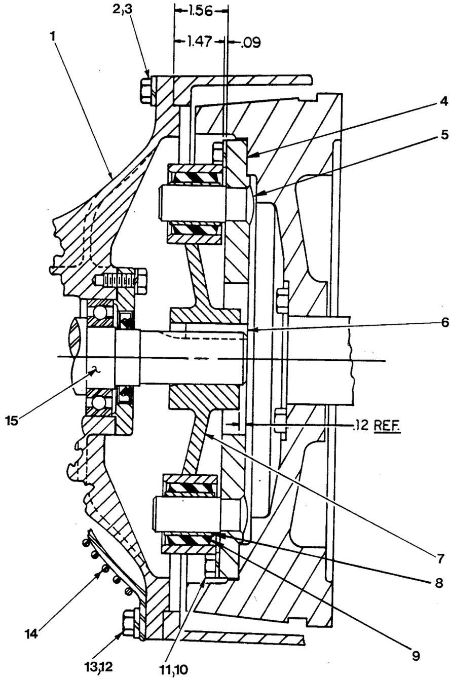
Figure 3. Drive Assembly For Pump Model 14C2-F3L
