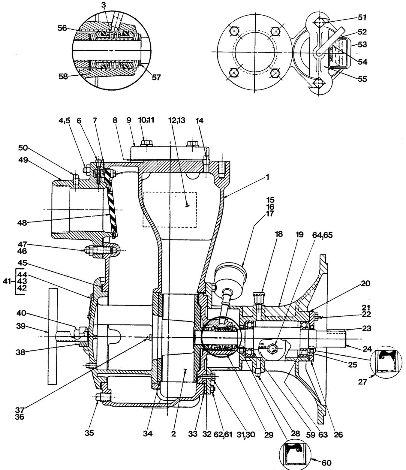
Figure 2. Pump End Assy 14C2-F3L
