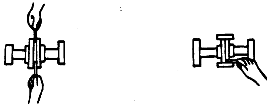
Figure 3B. Aligning Non-Spider Type Couplings
