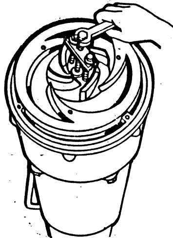
Figure 2. Removing Impeller With Puller
