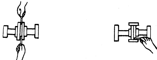
Figure 2B. Aligning Non-Spider Type Couplings
